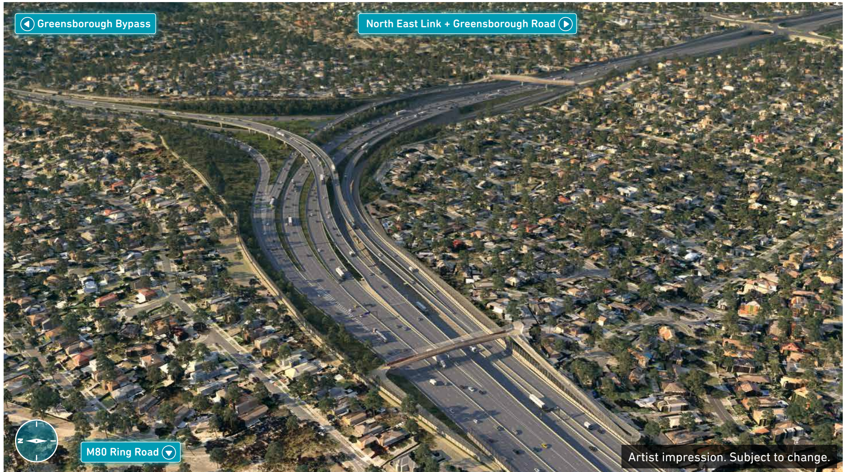
A free-flowing interchange connecting North East Link, the M80 Ring Road and Greensborough Bypass with Greensborough Road rebuilt on both sides of North East Link for local toll-free trips.
