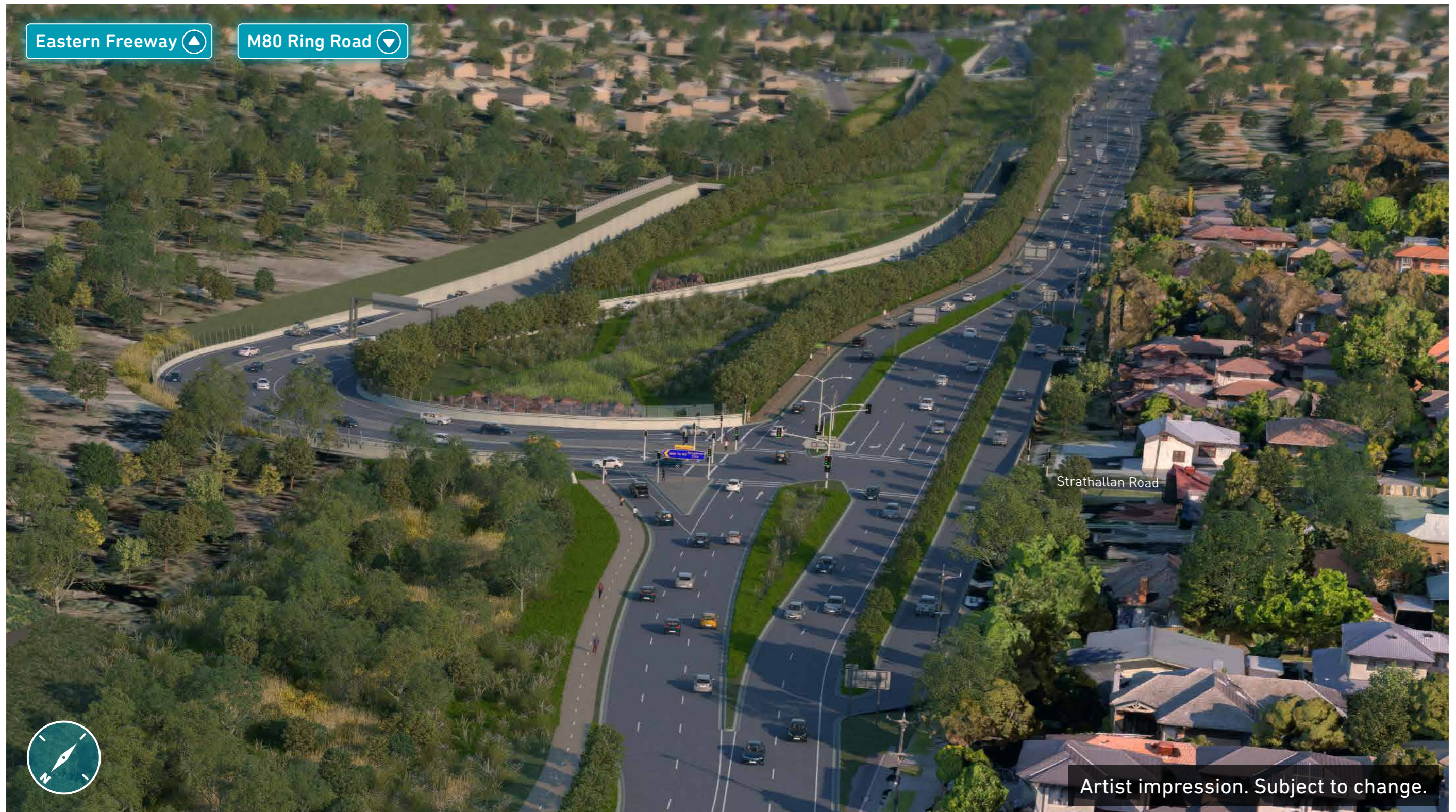
Entry and exit ramps in and out of the North East Link tunnels.
