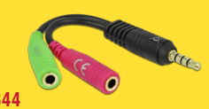
65344 Headset Adapter 1 x 3.5 mm 4 pin Stereo jack male to 2 x 3.5 mm 3 pin Stereo jack female (OMTP) 10 cm
