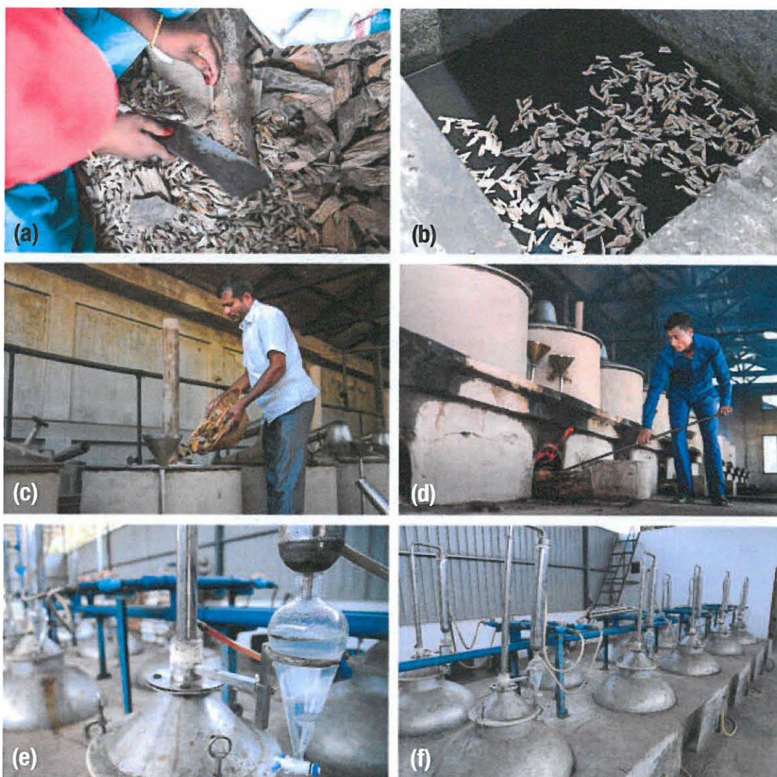
F-9 Summary of hydro distillation process for agarwood essential oil: (a) Wood chopping, (b) wood chip soaking, (c) filling of extraction pot, (d) boiling wood chips in water, (e) separation of oil using separating funnel and (f) example of semi-modern distiller.
