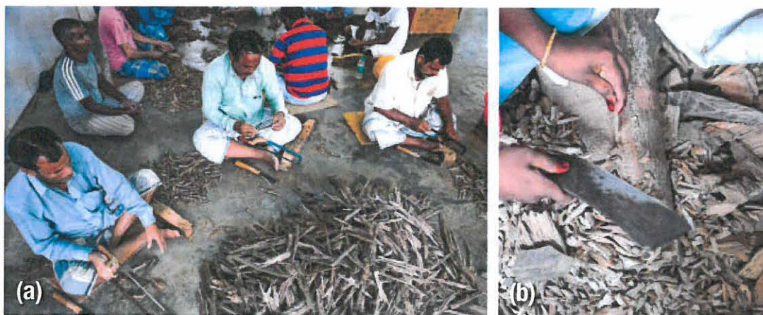
F-12 Woodchip of different qualities; (a) Woodchips with high resin content are sorted accordingly, (b) Inferior quality wood chips are chopped for extraction process.
