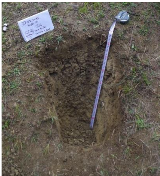
Photo 9: Soil profile of Rendzina with Ai horizon of only 5 cm (J. Etzold)
