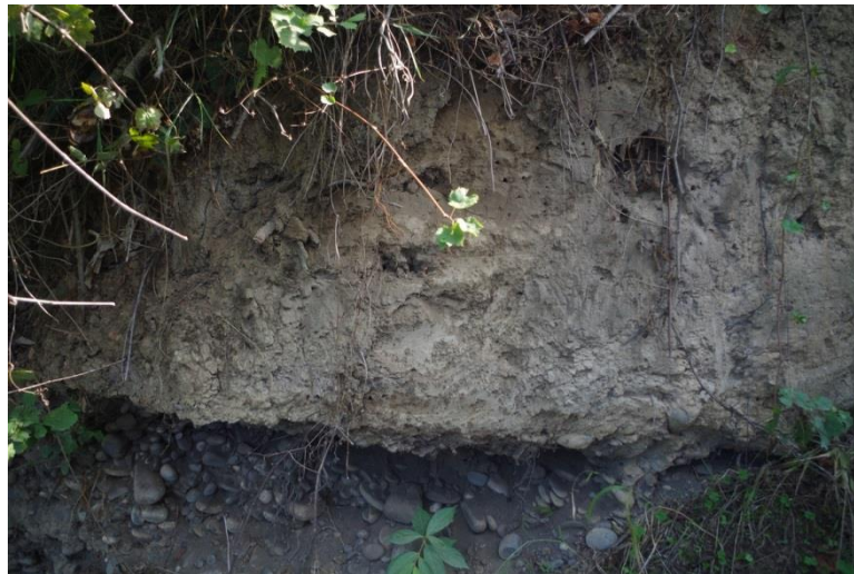
Photo 3: Cliff near the Caspian Sea showing the main texture of the region's soils: Aeolian sediments (loess) located on top of fluvial sediments (gravel and sand) (J. Etzold).
