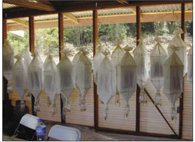
Set of mini-Winkler extractors, Nassau.
