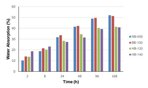
Fig. 3. The water absorption after the bleaching and heat treatment
