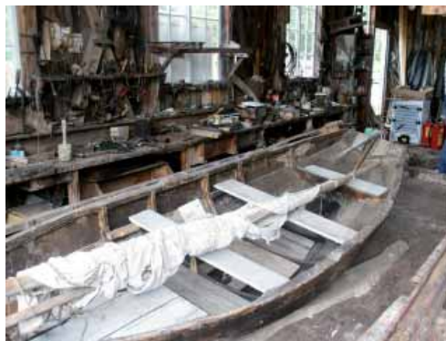
The Blekinge open rowing-boat was between 22 and 30 foot long and had a crew of 4 to 6 people. Usually it was sailed but in calm weather the crew had to row.
