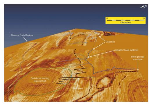
Figure 3.20 A salt dome at the west end of the Outer Silver Pit. Note that the river respects the dome, suggesting it was an upstanding feature
