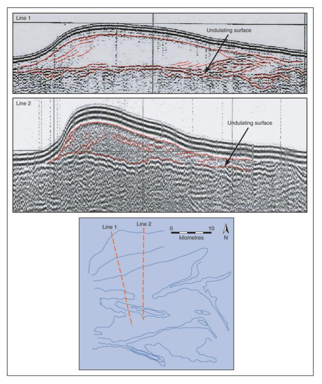
Figure 3.28 High-resolution slice across one sand bank showing that the underlying surface is highly irregular and possibly scoured by strong currents
