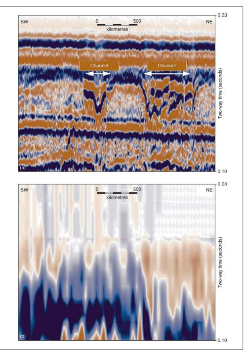
can be converted into an approximate depth and the continuous record built up into a profile through the Earth's surface. Typically, a vessel towing an acoustic source collects seismic data through a series of hydrophones designed to record the reflection from the seabed.
