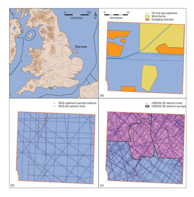
Figure 3.1 Detail of industrial activity in a small sample area west of the NSPP study area, including core positions and 2D and 3D seismic data
