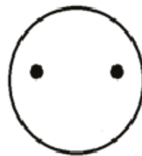
Fig. 1. The distribution of Whatman filter paper disks ( \Phi = 6 mm) impregnated with EO in the Petri plates
