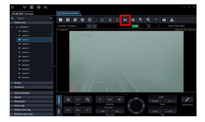
Select "Fog and Mist" in the "Correction mode" section on the visibility enhancement window.
