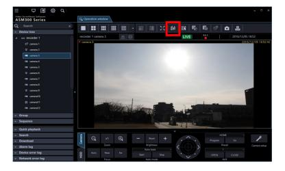
Select "Backlight" in the "Correction mode" section on the visibility enhancement window.
