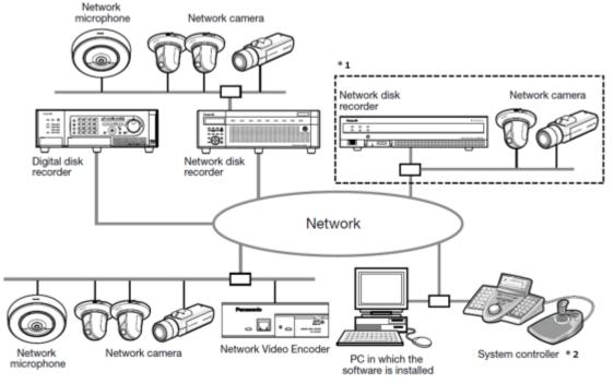
\*1 When a system that is surrounded by the dash-lines in the above diagram is configured, it is possible to directly monitor images from cameras that is connected to recorders without processing through recorders. In this case, check and set the following items.
