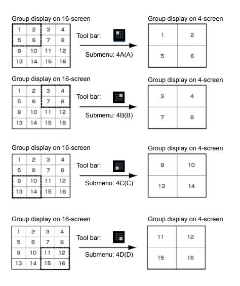
When the screen pattern is switched from 64-screen to 4A-screen, 4B-screen, 4C-screen or 4D-screen, images to be displayed will be as follows.
