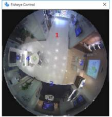
On this screen, it is possible to change the position to display using the correction function. By dragging and dropping a number icon of a screen whose display position is to be changed, that position will be the center of display.
