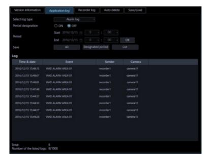
Click the desired button ([All] button/[Designated period] button/[Listed] button) according to the desired saving method of logs.
