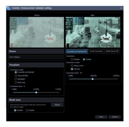
Adjust the parameters on each tab page of "Snowfall and Rainfall NR", "Spatial Tonal Correction" and "Multi-frame NR" of the visibility enhancement setting window. Descriptions about each parameter are provided on "Parameter list table".
