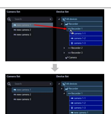
• When dragging a camera in the camera list and dripping onto "Independent camera folder" in the device list, the camera will be registered as an independent camera.
