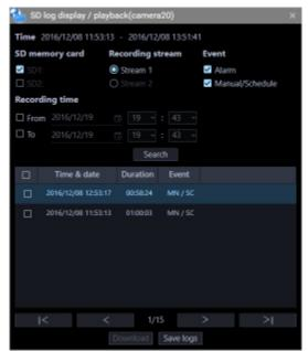
Set the display condition ("SD memory card", "Recording stream", "Event", "Recording time") in the "SD log display/playback" window, and click the [Search] button.
