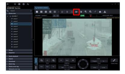
Select any of "User setting 1" - "User setting 4" in the "Correction mode" section on the visibility enhancement window.
