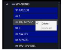
• When dragging a camera in the camera list and dripping onto a recorder in the device list, the camera will be associated with the first available channel of the recorder.
