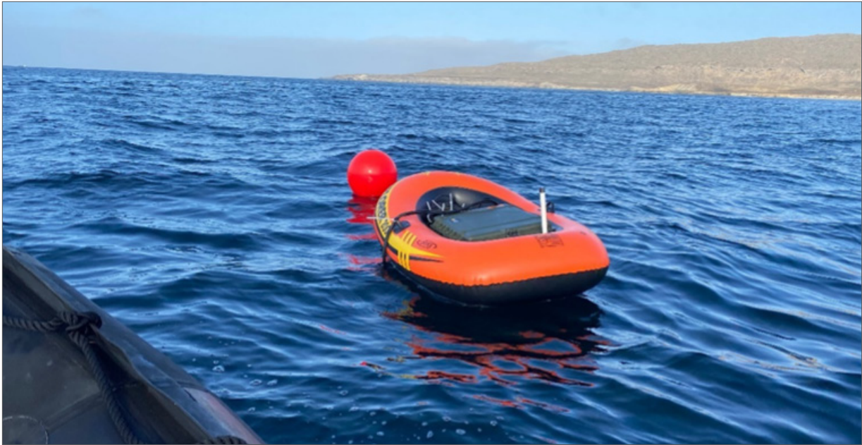
FIGURE 7-5: NSMRL's Aquarius sensor node was deployed in the raft and anchored at a measurement location during the Mine Neutralization Exercise 2020 trials.
