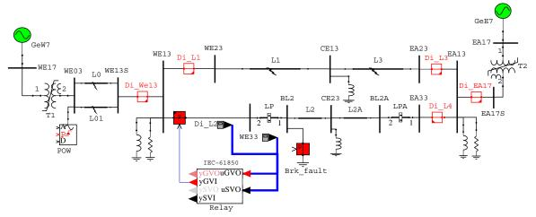
Figure 6: Power transmission network
