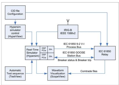
Figure 2: Hypersim simulator configuration for IEC 61850 test setup
