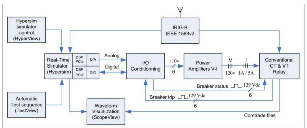
Figure 1: Hypersim simulator configuration for conventional CT & VT relay
