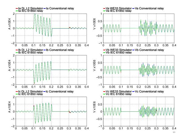
Figure 7: Voltage and current comparison between conventional and IEC 61850 relay
