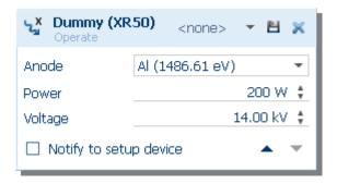
5. Enter desired values for the source power and high voltage as necessary.
