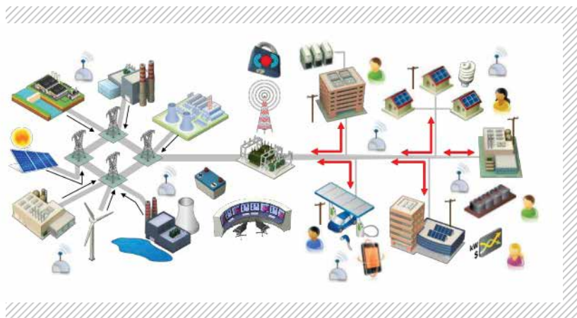
FIGURE 1: Tomorrow's power grid will have many components distributed over a large geographic area on both the supply and demand side. Rather than processing all information at the central control center, distributed solutions will provide scalable, large-scale coordination of the many active points in the grid. Image courtesy of Electric Power Research Institute (EPRI).
