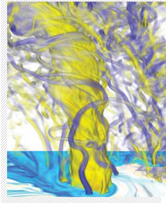
FIGURE 3: Vorticity field of the 20 meter simulation towards the end of the tornado's lifecycle. At this stage, the tornado has widened and taken on a multiple vortex structure.
