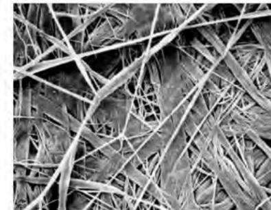
DuPont™ Tyvek® is a nonwoven, nonperforated sheet of spunbonded high-density polyethylene (HDPE) with microscopic pores large enough for moisture vapor to pass through, but small enough to resist air infiltration and water intrusion. The unique combination of properties – air infiltration resistance, bulk water resistance and vapor permeability—help protect a home from the elements, improve energy efficiency and prevent moisture from accumulating in walls.
