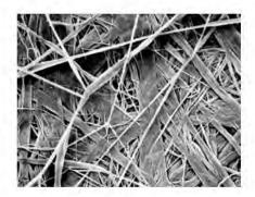
DuPont<sup>™</sup> Tyvek<sup>®</sup> is a nonwoven, nonperforated sheet of spunbonded high-density polyethylene (HDPE) with microscopic pores large enough for moisture vapor to pass through, but small enough to resist air infiltration and water intrusion. The unique combination of properties – air infiltration resistance, bulk water resistance and vapor permeabilityhelp protect a home from the elements, improve energy efficiency and prevent moisture from accumulating in walls.
