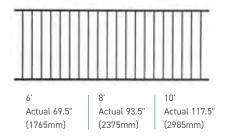
1" (254mm) wide 16 GA top & bottom rail 5/8" (159mm) wide 16 GA baluster 3-7/8" (984mm) between balusters
