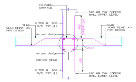
Fig. 15 Roof Slab & outer wall connection
