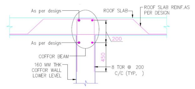
Fig. 16 Roof Slab & Inner wall connection
