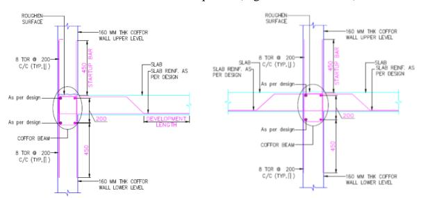
Fig. 13 Slab & outer wall connection
