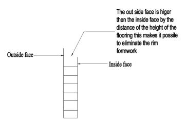
Fig. 11 Adopting the formwork to the wall height
