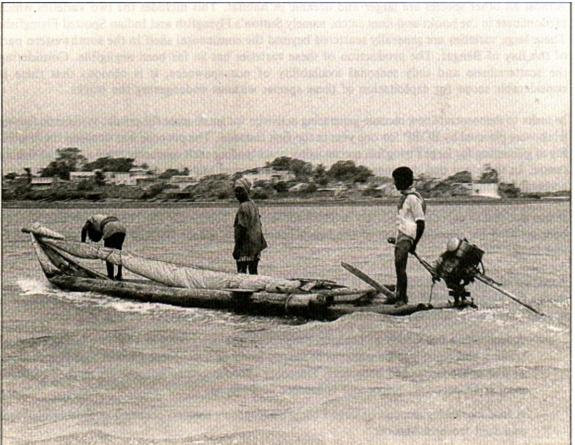
A large kattumaram in Thirumullaivasal, one of the few with an engine (a longtailed diesel engine)
