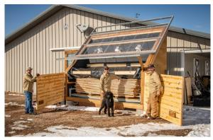
A solar kiln to dry lumber to desired moisture content for CLT fabrication (photo courtesty of TimberAge Systems)
