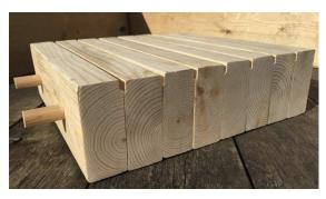
Figure 5. Dowel-laminated timber sample. Photo courtesy of Fast+Epp (https://www.fastepp.com/concept-lab/material/dowel-laminated-timber-dlt-4/)
