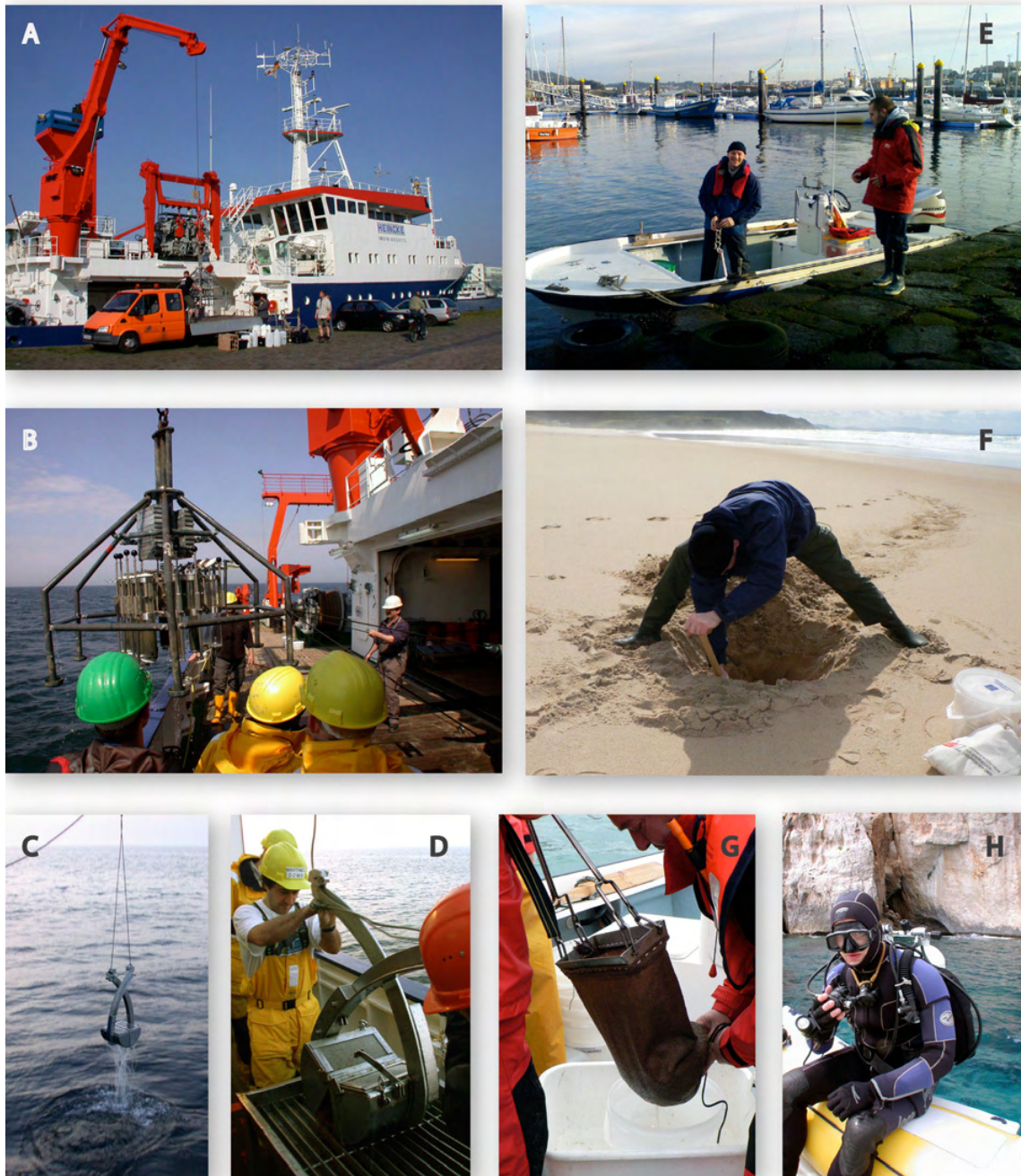
Figure 2.1: Some impressions of the field and species collection work. A shows the FS Heincke (Alfred Wegener Institut, Bremerhaven), a German research vessel before joining an offshore trip of several days on the North Sea. B : the Multicorer is lifted on deck. C – D : the Van Veen grab sampler coming up ( C ) and its opening to sort the samples ( D ).
