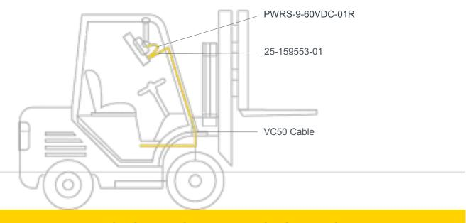
VEHICLE MOUNT (WHEN REPLACING THE VC50 AND REUSING THE VC50 DC POWER CABLE)
