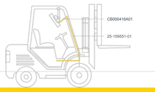
VEHICLE MOUNT (WHEN REPLACING VC70 AND REUSING THE VC70 DC POWER CABLE)
