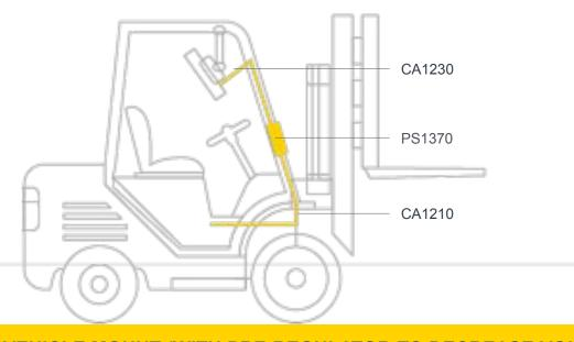
VEHICLE MOUNT (WITH PRE-REGULATOR TO DECREASE VOLTAGE - FOR TRUCKS WITH BATTERIES GREATER THAN 48V)
