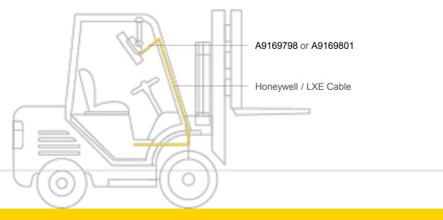
VEHICLE MOUNT (WHEN REPLACING A HONEYWELL/LXE VC AND REUSING THE DC POWER CABLE)
