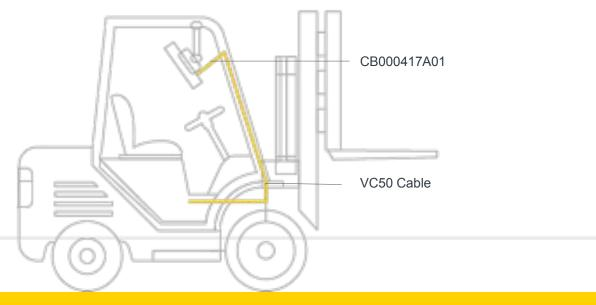
VEHICLE MOUNT (WHEN REPLACING VC50 AND REUSING THE VC50 DC POWER CABLE)
