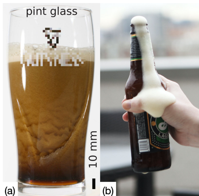
FIG. 12. Examples of dynamic and unstable foaming phenomena. (a) Unique foamy textures in stout with nitrogen bubbles. From Watanura et al. , 2021. (b) Foam overflow “volcano” due to tapping on a beer bottle. Public domain image.
