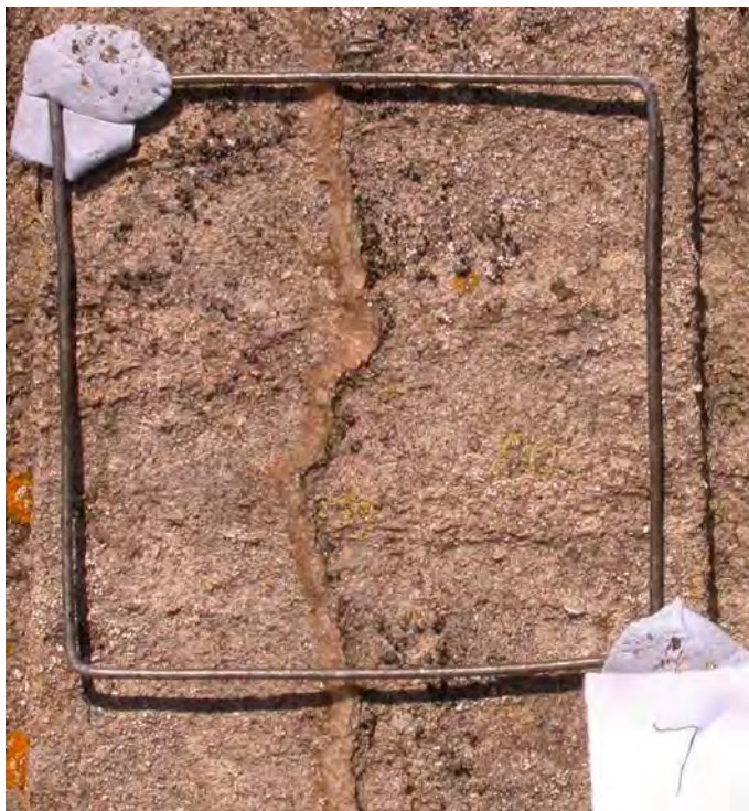
Figure 6. Lichen Community at sample point 7 1.1m from base of the tower of St Stephens Church, Bath.
