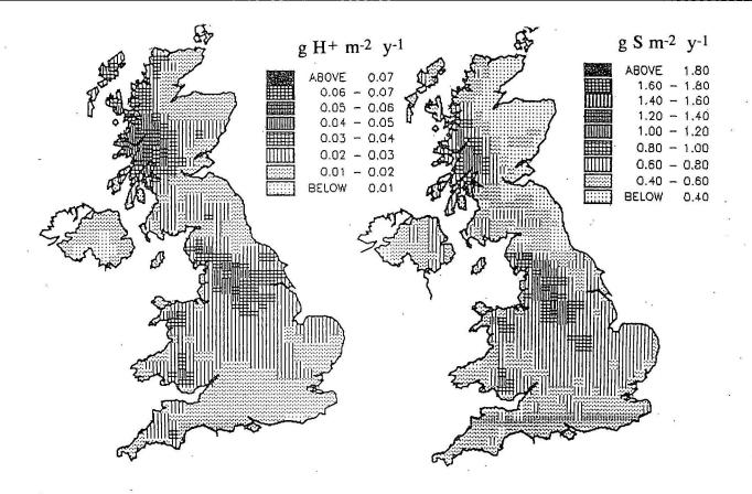
Fig 4. Geographical variation in wet deposited hydrogen ions and non marine sulphate in 1989 (Campbell, Stedman & Irwin (1992), Warren Spring Laboratory].
