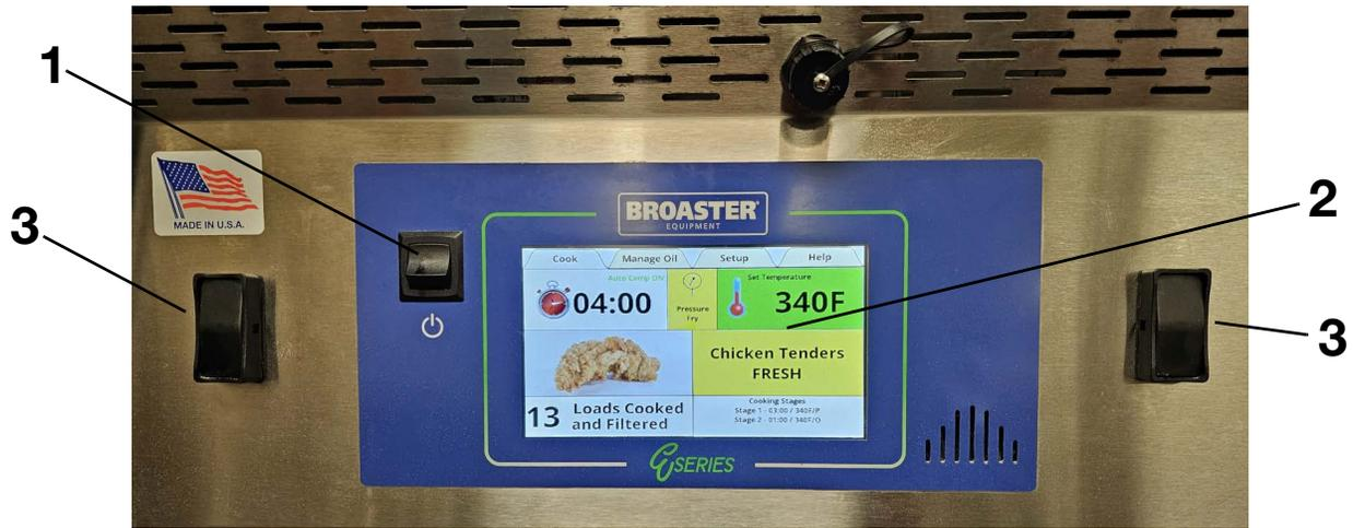
**1. Power Switch:** This switch has two positions: ON (UP) or OFF (DOWN).
