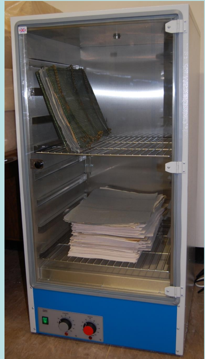
Drying oven with air circulating, 30 degrees
