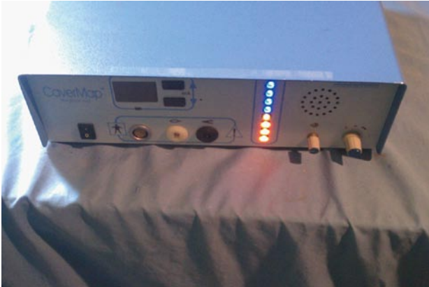
Figure 5 The CaverMap Surgical Aid nerve stimulator control unit. Device control unit with connectors for the stimulation needle, display of the applied current in mA, and light-emitting diode display (blue and red) to visualize tumescence response on an ordinal scale.
