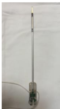
Figure 1 Trans-urethral ultrasound therapy probe. Rigid, water-cooled trans-urethral ultrasound applicator with 5 mm (15 French) diameter and eight transducer elements (4 mm x 5 mm/element).
