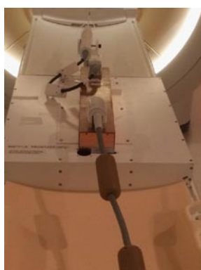
Figure 2 Magnetic resonance imaging-compatible ultrasound therapy device. Set-up of the trans-urethral ultrasound applicator on the MRI patient table with control cables, and motor unit to control the rotation of the ultrasound transducer. MRI: Magnetic resonance imaging.
