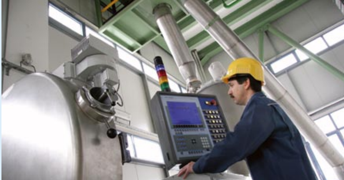
Rigid granule producing extruder in the Granulating Plant
