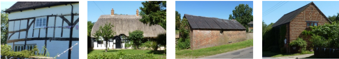
Timber frame and render, hipped thatch, brick with slate roof and decorative brickwork
