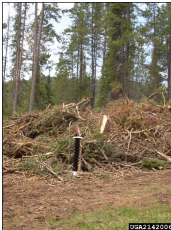
Figure 6. Lundgren funnel trap used to detect pine engraver beetles at a slash pile. (Brytten Steed, USDA Forest Service, Bugwood.org)
