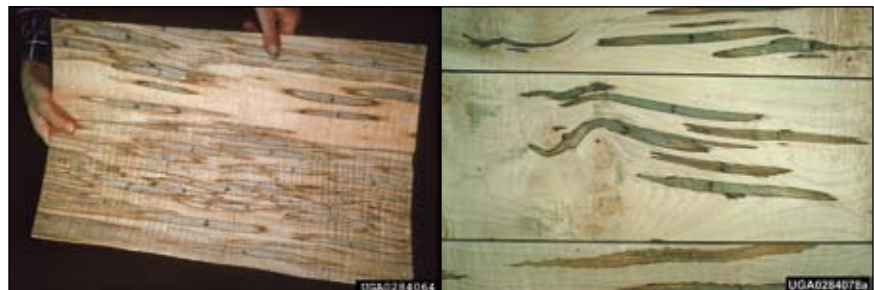
Figure 5. Milled maple timber shows the callus-filled galleries of Columbian timber beetle, and blue staining of associated ambrosia fungus. (Left: Jack C. Nord, USDA Forest Service, Bugwood.org; right: James Solomon, USDA Forest Service, Bugwood.org)
