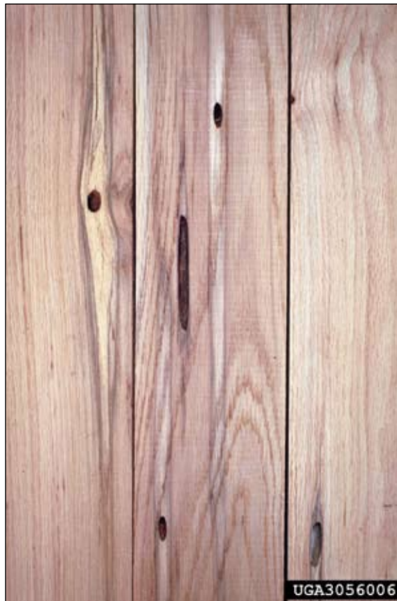
Figure 7. Defects in milled wood from carpenterworm tunnels and staining. (James Solomon, USDA Forest Service, Bugwood.org)
