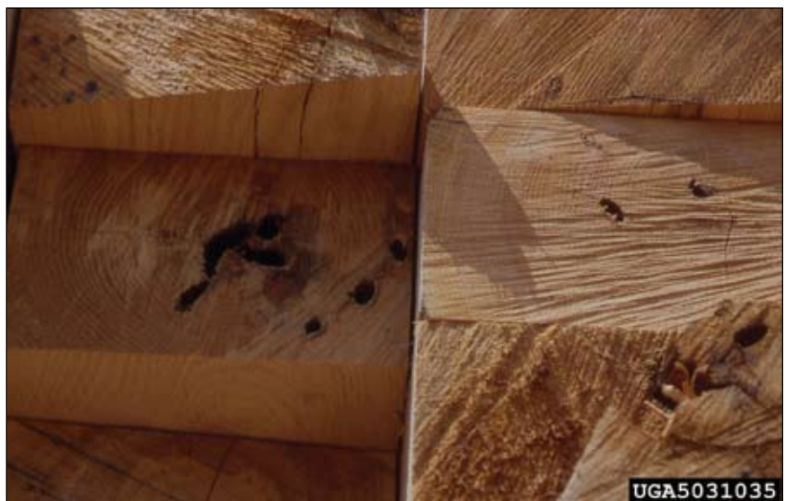
Figure 9. Lumber cut from infested trees is downgraded because of the galleries of red oak borer. (Joseph O'Brien, USDA Forest Service, Bugwood.org)
