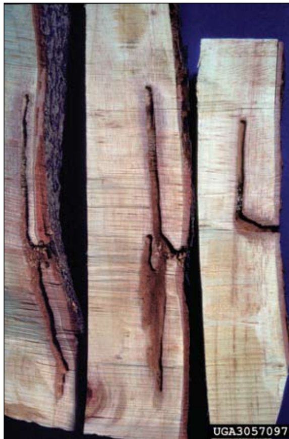
Figure 4. Larval tunnels of pecan carpenterworm seen in longitudinal section in pieces of milled wood. (James Solomon, USDA Forest Service, Bugwood.org)
