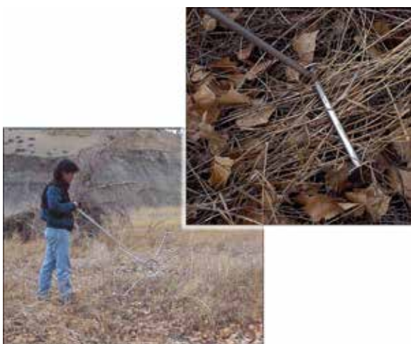
Figure 82. Wheel sampler used in vegetation monitoring. AAFC.
