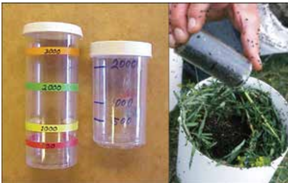
Figure 65. Plastic vials developed to volumetrically estimate numbers of collected Aphthona spp. adults. USDA-APHIS.
