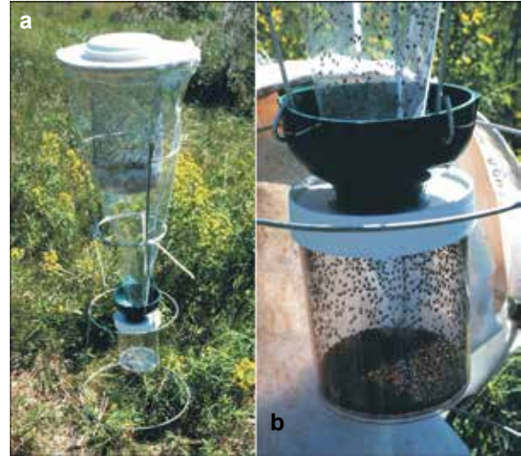
Figure 64. The “ Aphthona accelerato ” flea beetle sorter developed by TEAM Leafy Spurge. (a) the sorter as used in the field; (b) the collecting container at the bottom holding A. lacertosa adults. USDA-APHIS.
