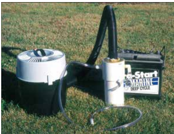
Figure 61. Small collecting vacuum that is powered by a 12-volt car battery and used to sort Apthona adults under field conditions. USDA-APHIS.
