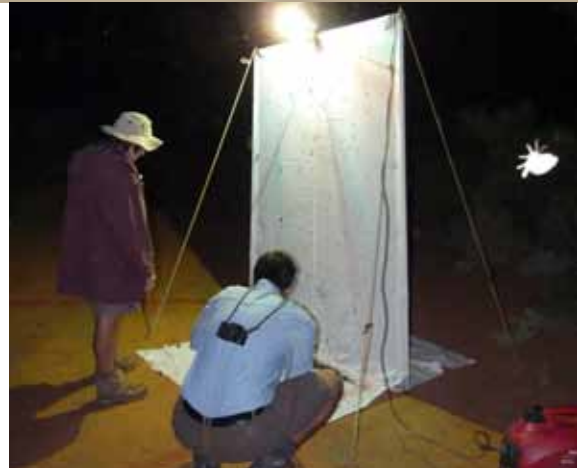
A mercury vapour light trap, used to catch nocturnal flying insects © Copyright, Queensland Museum
