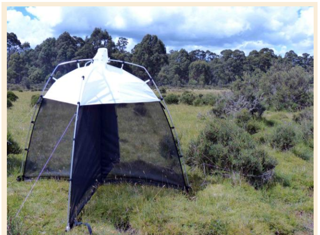
A SLAM trap, designed to trap insects that fly up after hitting a barrier, photo Simon Grove © copyright, TMAG
