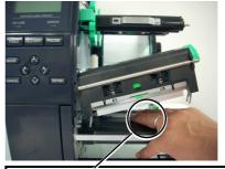
Care must be taken not to allow a metal object like a ring to touch the print head edge.
