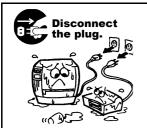
If foreign objects (metal fragments, water, liquids) enter the machine, turn off the power switch and disconnect the power cord plug from the outlet, and then contact your authorised TOSHIBA TEC representative for assistance. Continued use of the machine in that condition may cause fire or electric shock.
