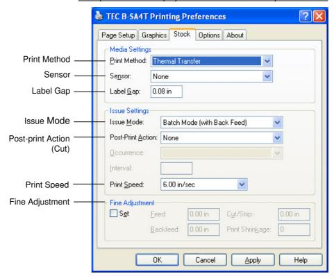
Print Method: Direct thermal or thermal transfer is selectable.
