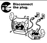
Continued use of the machine in an abnormal condition (the machine is producing smoke or a strange smell) may cause **fire** or **electric shock**. In these cases, immediately turn off the power switch and disconnect the power cord plug from the outlet. Then, contact your authorised TOSHIBA TEC representative for assistance.
