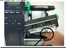
Care must be taken not to allow a metal object like a ring to touch the print head.
