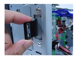
1.2. Attach the Cover to the printer back with the two M-3x6 screws, as shown below.
