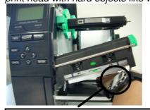
Care must be taken not to allow the metal or glass part of a watch to touch the print head.
