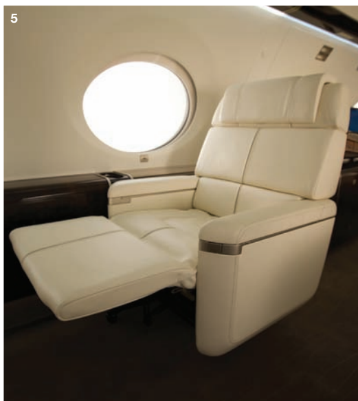
4-6. Two of the G650’s standard seats are electrically operated, and feature heated back and base cushions; four-way pan tilt; back cushion massage; single-position memory preset; and press-and-hold controls for full upright and full-flat positions
