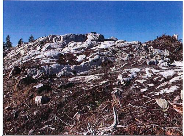
Photo 2 – Typical strong dioritic bedrock with widely spaced discontinuities at Denny Island MCTS site
