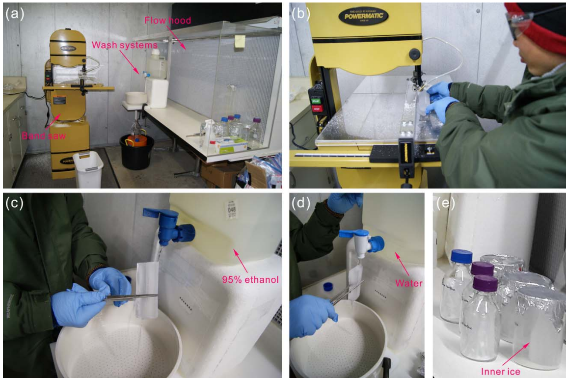
Supplementary Figure S1 Ice core sampling and preparation in the laboratory. (a) The cold work room ( -5^{\circ}\text{C} ) with band saw, BioGard laminar flow hood and wash systems. (b) the outer layer of the ice section being removed by the band saw. (c) The ice section being washed with 95% ethanol and (d) with water. (e) The “clean” inner ice is preserved in the autoclaved beakers or bottles.
