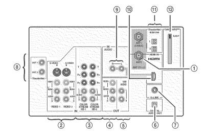
1 ANT-1 (CABLE) IN and ANT-2 IN — Two inputs that support analog (NTSC) and digital (ATSC) off-air antenna signals and analog and digital (QAM) Cable TV signals.
