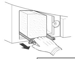
Note: Wear gloves when replacing the lamp unit.
