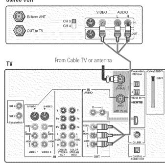
**Note:** The VIDEO/AUDIO OUT jacks output the signals from the ANT 1, ANT 2, VIDEO 1, VIDEO 2, or VIDEO 3 jacks when the appropriate input mode is selected.
