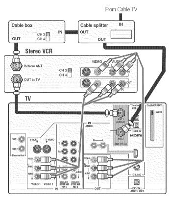
**Note:** The VIDEO/AUDIO OUT jacks output the signals from the ANT 1, ANT 2, VIDEO 1, VIDEO 2, or VIDEO 3 jacks when the appropriate input mode is selected.
