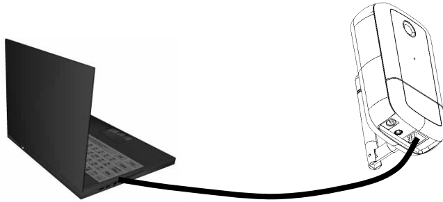
① CAT 5 Ethernet cable
