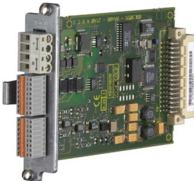
Figura 4-43 Terminal Board TB30
