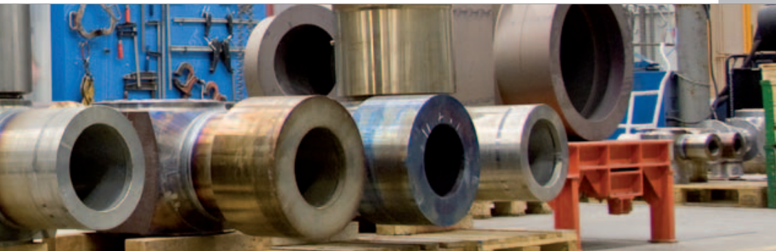
Inspection of welded components for high-pressure valves
