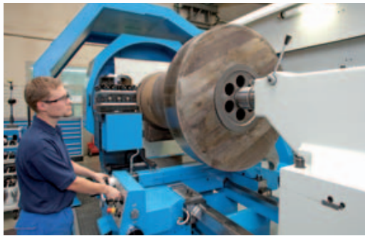
Machining a boiler circulating pump casing
