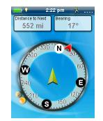
The Compass screen displays a recognisable compass that can be used to display your heading and your heading's relation to the sun, moon and your destination (red arrow). The data fields at the top of the display are customisable (see *Customising the Data Fields*). The graphic displayed that is used for the compass is customisable as well.
