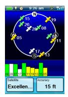
The Satellite Status screen displays a graphical representation of the satellites overhead in relation to you current location (the centre of the circle). The colour of the satellite graphics, as well as the bar graph, indicate the signal strength of the signals being received. The numbers indicate the assigned satellite designation. The data fields at the bottom of the display are customisable (see *Customising the Data Fields*).
