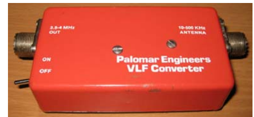
Fig. 5, A commercial VLF converter, up-converting to 4 MHz. Paul Shinn used such a converter to capture SAQ.
