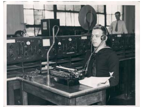
Fig 14: The Navy long wave receiving station in the Washington, DC area, 1930s; Navy RE, RF & RG receivers.
