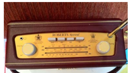
Fig. 29: A modern English "Roberts" portable radio covering long wave as well as AM and FM. (Author's collection, from Alan Carter, BVWS).
