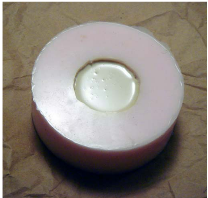
Fig. 8: Resin curing in the mold.
