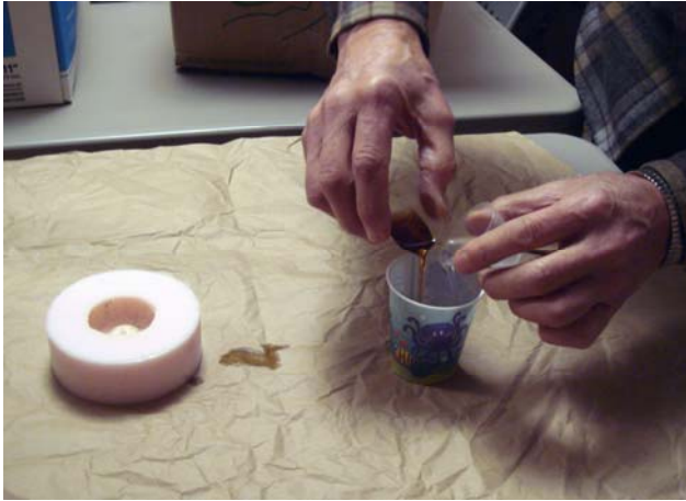
Fig. 5: Pouring the two resin chemicals A & B into a cup.
