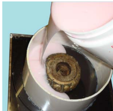
Fig. 3: Pouring the mold compound.
