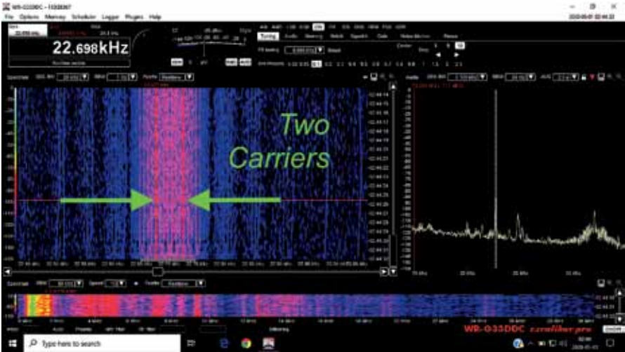
Fig. 41. The signal's bandwidth grows to 800 Hz with two internal carriers at 02:44 UTC. (Author's screen cap)
