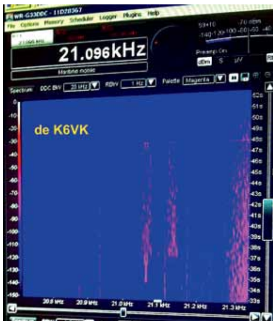
Fig. 21. The Russian worldwide VLF station RDL on 21.1 kHz, a screncap from the WinRadio G33 at K6VK. (Author’s photo)
