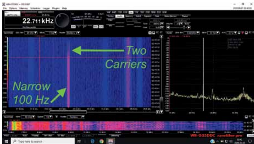
Fig. 40. This initial 22.7 kHz signal’s bandwidth may be 100+ Hz, early in the evening of May 1, 2020. This signal is stronger than NLK in Washington state (“Jim Creek”) at 24.8 kHz, bandwidth 200 Hz. (Author’s screen cap)
