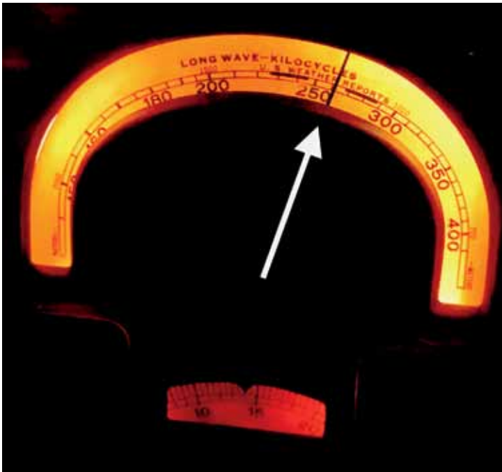
Fig. 25. The dial showing the “Weather Band” around 250 kHz, on a 1936 RCA 10K console radio. (Author's collection)
