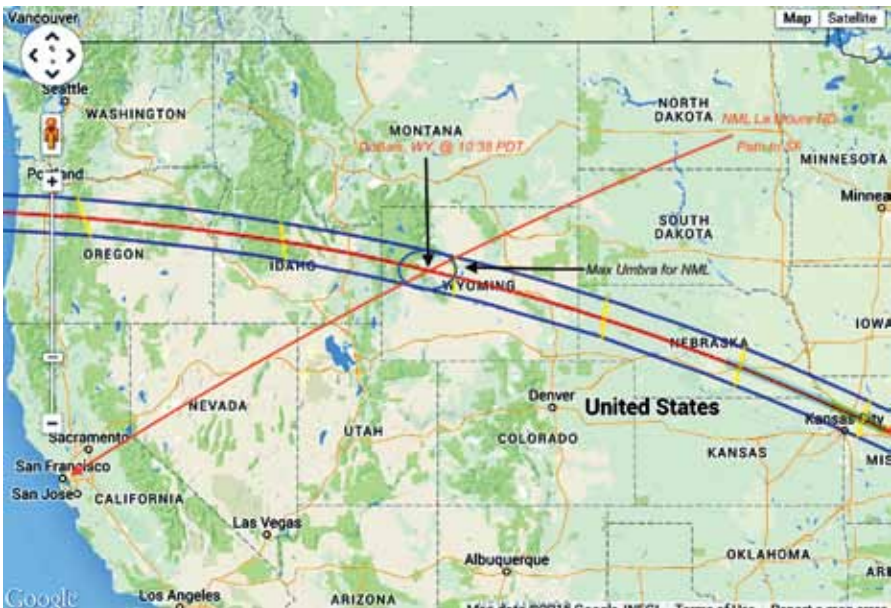
Fig. 45. The 2017 Solar Eclipse and VLF station NML signal at 25.2 kHz path Intersection.
