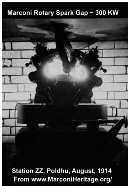
Fig. 6. A Marconi high power rotary spark gap in action August 1914 at 300 kW. (Image from MarconiHeritage.org)
