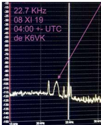
Fig. 43. The mystery signal as first logged at K6VK on November 8, 2019, at 22.7 kHz about 04:00 UTC (local late evening), on the WinRadio G33. (Author's screen cap photo)
