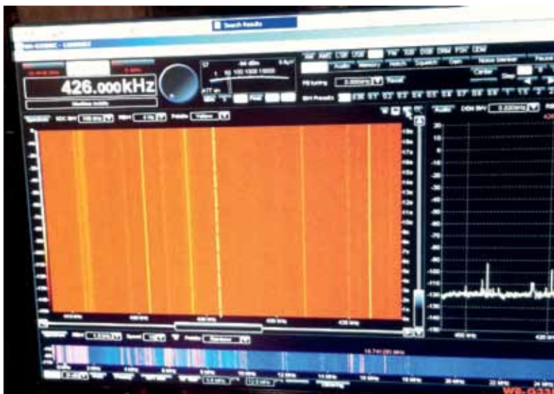
Fig. 36. Morse code from KSM at Bolinas on 426 kHz November 2, 2014, from the WinRadio G33 receiver at K6VK. (Author's screen cap photo)
