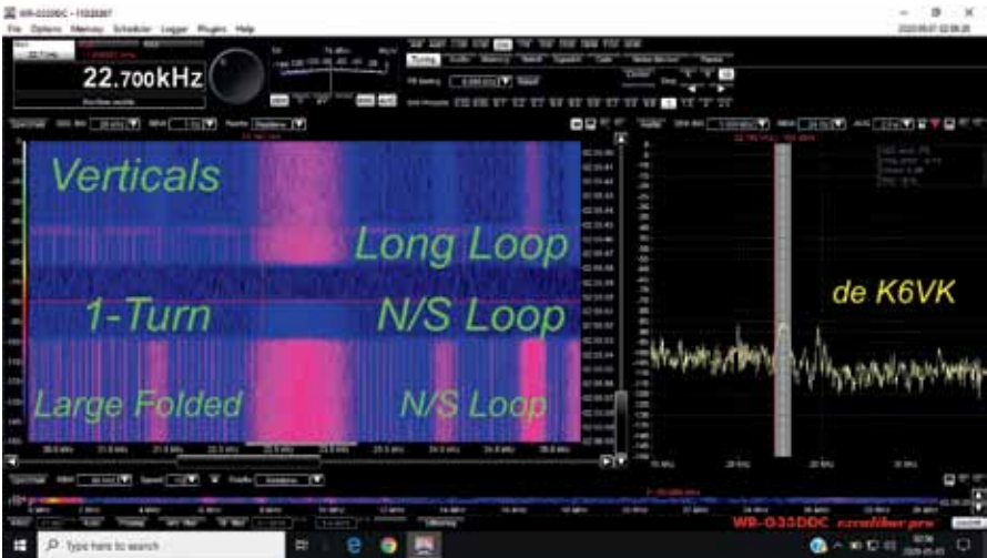
Fig. 42. The signal on 22.7 kHz at 02:56 UTC by way of four differentially directional antennas, the north-south VLFL loop was strongest at 46 microvolts on the WinRadio G33 at K6VK. (Author's screen cap)
