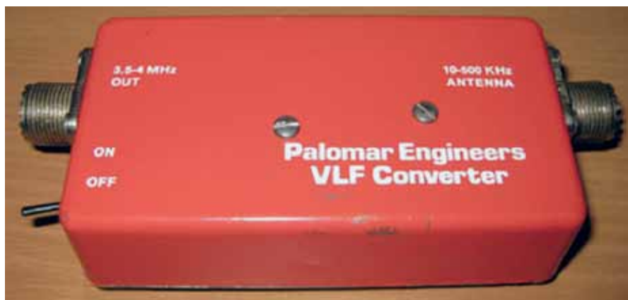
Fig. 5. A commercial VLF converter, where the 0–500 kHz band is up-converted to 3.5–4 MHz (80 meter ham band). Paul Shinn used such a converter to capture SAQ. (Internet sourced)
