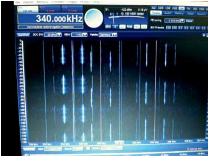
Fig. 24. Station CC in Contra Costa County, CA at 335 kHz, a typical LF beacon for an airfield. (Author's screen cap)
