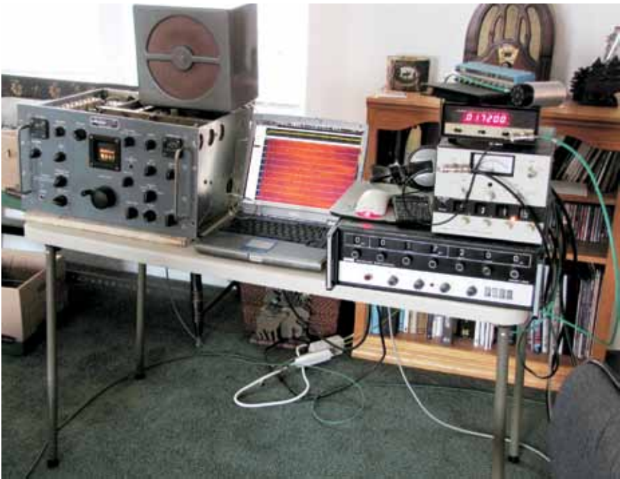
Fig. 1. The VLF receiving post of John Staples on Mt. Shinn, near Lodi, California in 2012, with his Collins R-389 VLF receiver. (John Staples)
