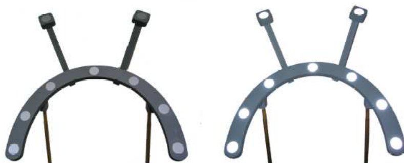
Figure 2.3: Fiducials without flash (left) and with flash (right)
