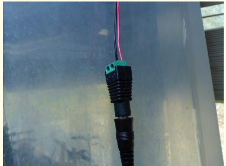
Connection between the fan and the adaptor. The positive (red) and negative (black) wires are easily inserted into the adaptor and tightened down with a small Phillips head screwdriver.
