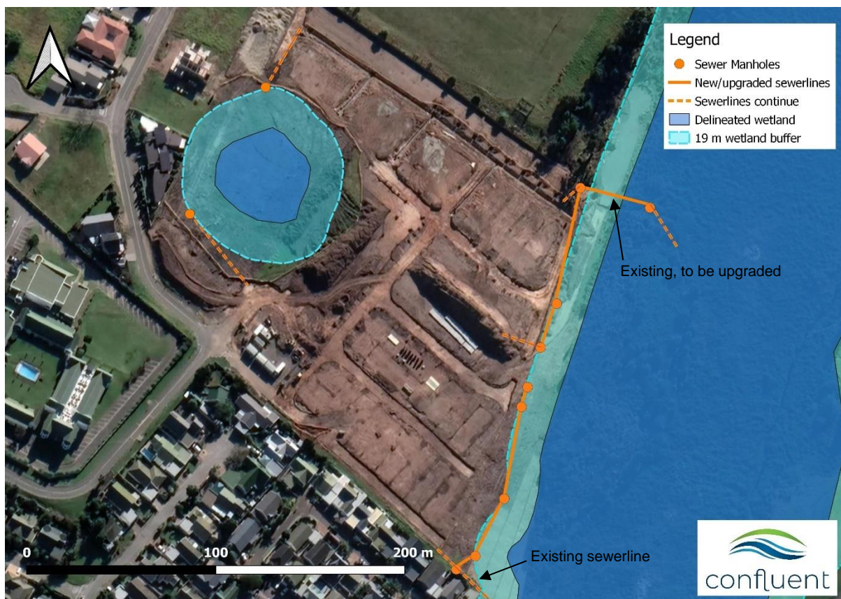
Figure 18. Mapped sewerlines and manholes for the Preferred Layout in direct proximity to wetland and buffer areas (Refer to Zutari Engineering Services report, 2022).
