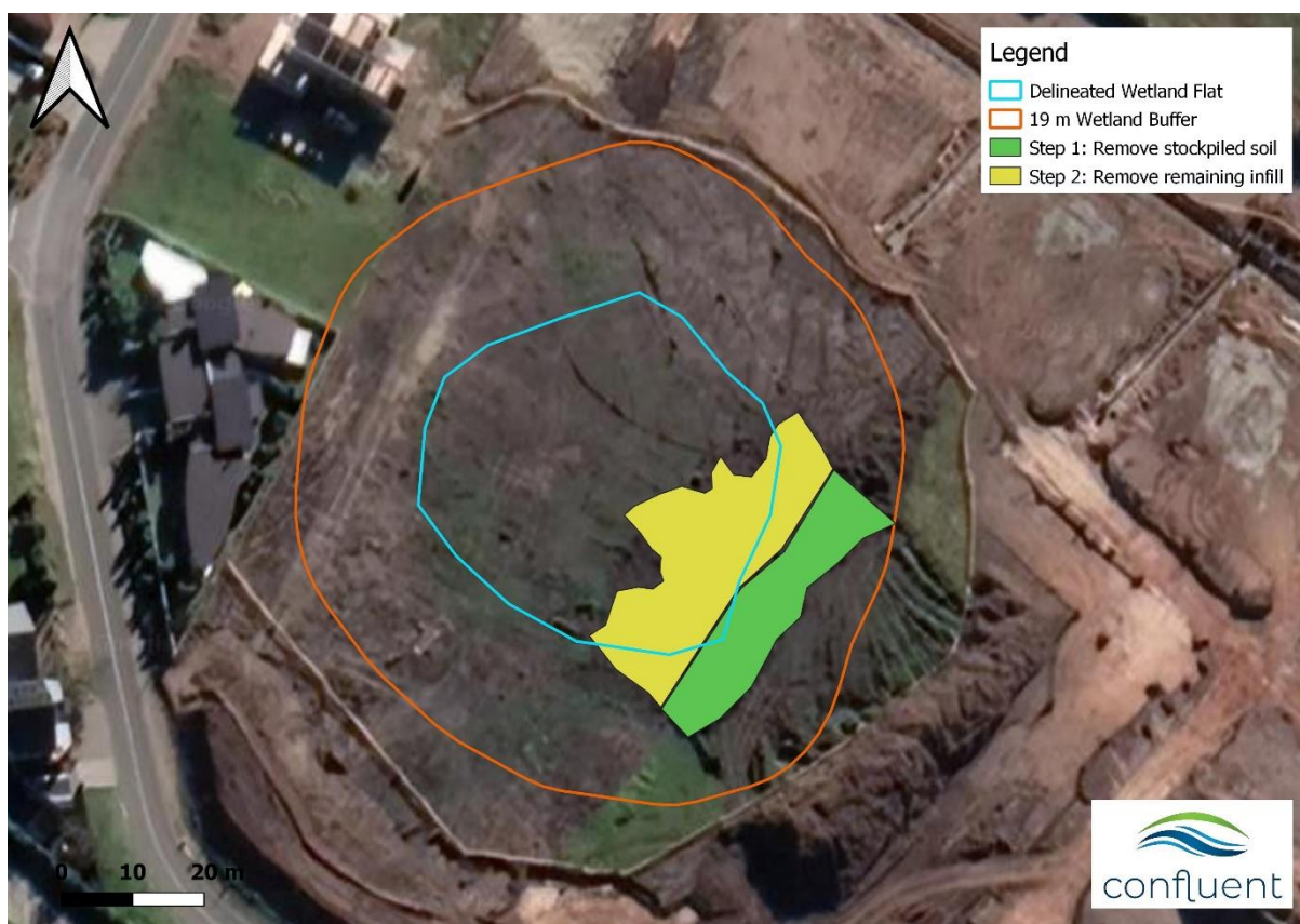
Figure 16. Map showing Step 1 and Step 2 soil to be removed from the Wetland Flat and buffer area.
