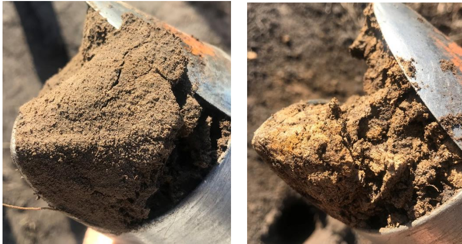
Figure 13. Example of augered soil down the slope towards Camphersdrift wetland showing soil with no wetland indicators (left) compared to soils with indicators of temporary wetness (right).
