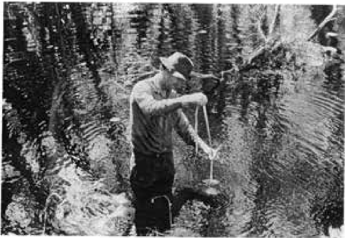
Plate 2. Measuring water clarity using a secchi disc. Black Creek, near Hope Vale.
