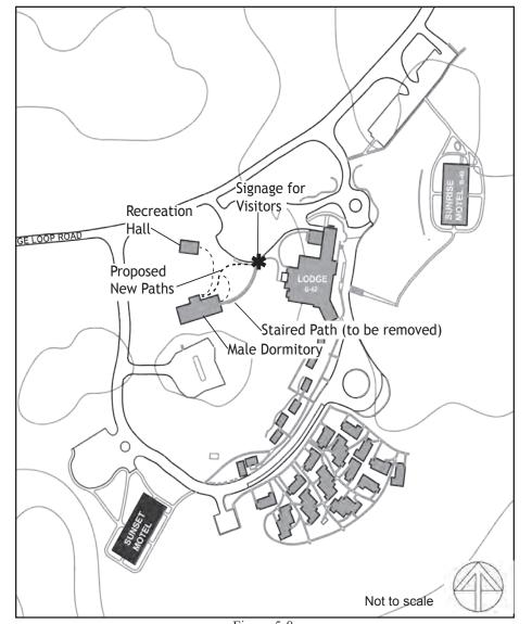
Figure 5-8. Proposed Realignment of the Path to the Male Dormitory.
