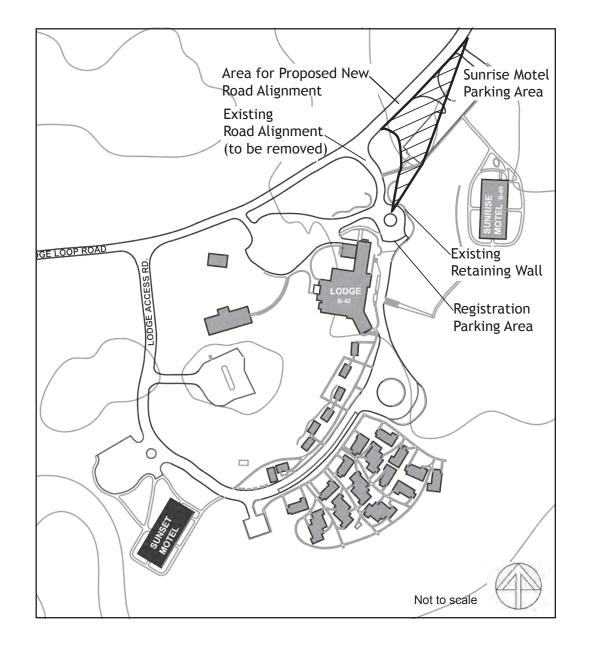
Figure 5-6. Proposed Realignment of the Lodge Access Road North of the Lodge
