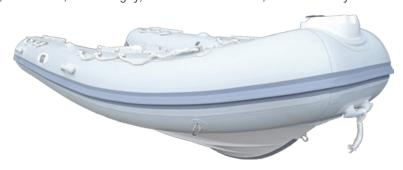
Designed to deliver the perfect balance of functionality and performance, HSF is impressive both at rest and on the move. The pronounced bow-sheer, deep V keel, large tube diameter and full-length lifting strakes of this series guarantees a great sea-going vessel and a smooth dry ride. Its stability at rest, its spacious cockpit and its heavy duty grab handles, makes the ideal platform as a dive boat, rescue/response boat or coach/support boat.
